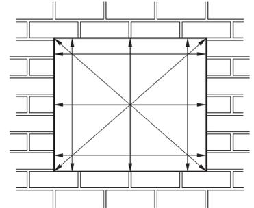
A window or door set with a check reveal it is a good idea to remove an internal architrave from the window or door set, to be see exactly how deep the reverse brick detail really is and to identify how much of the outer frame can be put behind in the width. A hole should be drilled through the head of the existing box frame to ascertain the maximum height the window or door set can be put behind the brick.
